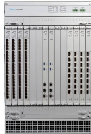
**ME5000M** routers are multifunctional devices with a high port density intended for use in provider networks as aggregation routers and IP/MPLS network edge routers. ME5000M is a cost-effective, reliable and high-performance solution which can be used to organize operator's points of presence when providing data services for large customers with high reliability requirements.
