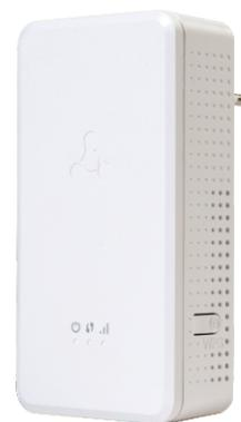
RR-11 is a wireless signal repeater designed to extend wireless networks coverage area and amplify Wi-Fi signal strength. The device helps to eliminate blind spots and optimize your Wi-Fi network operation.
