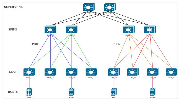
The IP fabric is divided into two PODs (see Terms and abbreviations), and an additional switching layer (SuperSpine or Second-layer Spine) is implemented. The diagram shows that the PODs are isolated from each other: the First-layer Spine (Spine\_11-22 in the diagram) only has connections to a specific group of Leaf devices that belong to its POD. PODs are connected to each other via the Second-layer Spine.
