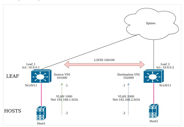
On Leaf\_1, a VXLAN with VNI 101000 and VLAN 1000 are created. The VLAN 1000 IP interface is added to VRF1 so that L3VNI is used to route client packets. Then and IP address is assigned to this IP interface.
