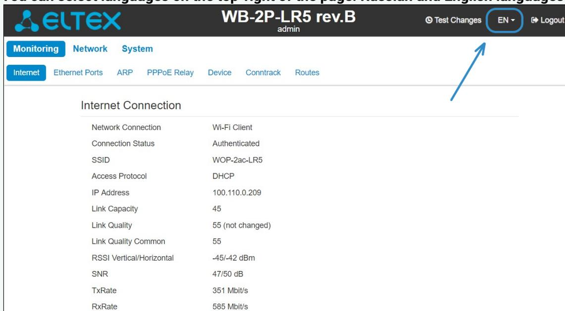
The screenshot shows the top navigation bar of the ELTEX WB-2P-LR5 rev.B web interface. The user is logged in as 'admin'. The language dropdown menu is set to 'EN' and is highlighted with a blue circle and an arrow. Below the navigation bar, the 'Internet' section is active, displaying the 'Internet Connection' status table.
