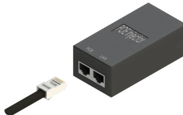
2. Connect Ethernet cable of your LAN network or PC to LAN port of PoE injector.
