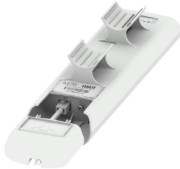
3. Connect Ethernet cable to LAN port.
