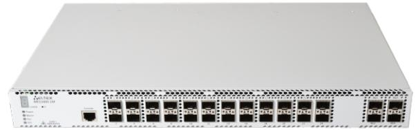
MES3400 new generation switches can be used in service provider networks as aggregation or transport switches. They ensure high performance due to the universal interfaces operating at speeds of 10 Gbps or 1 Gbps. The benefits of MES aggregation switches include advanced L2 functions, support for static and dynamic routing, hot-swappable redundant power modules.
