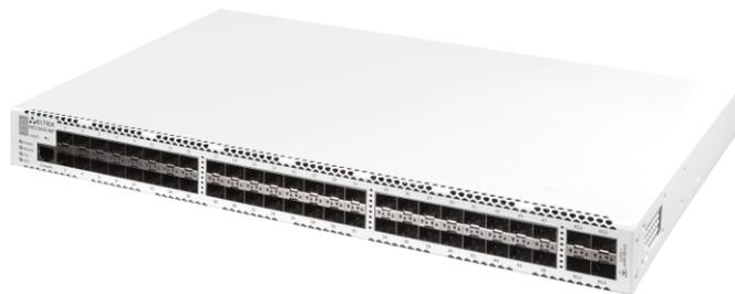
The new generation switches MES3400-48F can be used in service provider networks as aggregation or transport switches. They ensure high performance due to the interfaces operating at data rates of 10 Gbps or 1 Gbps. MES aggregation switches' feature set includes advanced L2 functions, static routing, dynamic routing, redundant and hot-swappable power supplies.
