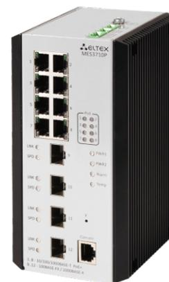
**MES3710P** industrial switches manufactured by ELTEX are designed to organize fault-tolerant networks on sites with high requirements to temperature, vibrations and mechanical impact. The switches have 10/100/1000BASE-T ports with PoE/PoE+ technology support and 100BASE-FX/1000BASE-X (SFP) ports.
