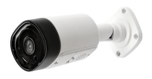
**SV-BA301-E** wired IP camera with a cylindrical design provides a horizontal viewing angle of  $100^{\circ}$  and is equipped with a 4 MP CMOS matrix for clear video with a resolution of up to  $2560 \times 1440$ . The device has a night shooting mode (IR illumination), motion detection system and the function of saving the video archive to a memory card or network storage<sup>1</sup>. The camera is equipped with an RJ-45 connector with support for basic network protocols.
