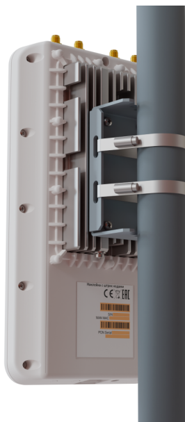
Figure 9 — Attaching the device to the pole
