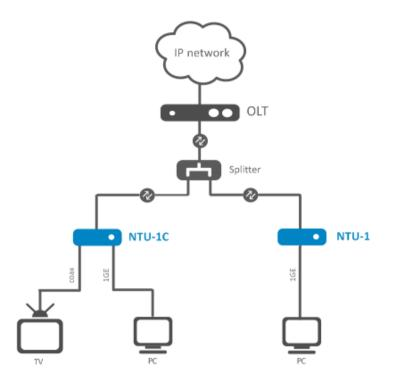
Figure 1 – Connection of NTU-1, NTU-1C
