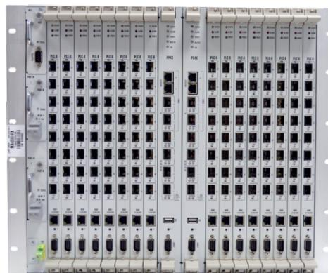
Multi-service access and aggregation node MA4000-PX is dedicated for access networks based on GPON technology. The OLT allows operators to construct scalable, fault tolerant "last mile" networks meeting high safety requirements in either urban or rural areas. MA4000-PX controls customer equipment, traffic switching and access to transport networks.
