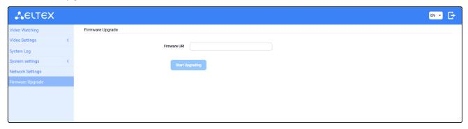
$\cdot$  Firmware URI — URI link that allows the camera to download the firmware for upgrading. Click the "Start Upgrading" button to start the upgrade.
