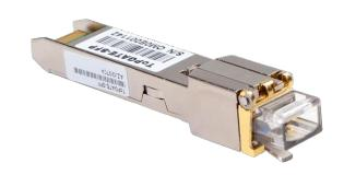
PPP connection is established between the routers, through which traffic is transmitted. When the connection is established, the ToPGATE-WAN-E1 module can use part of DS streams (64 Kbps), combining several streams to the desired bandwidth, i.e. the transmission rate can be adjusted from 64 Kbps to 2048 Kbps. ToPGATE-WAN-E1 module supports G.703 standard and HDB3/AMI encoding.
