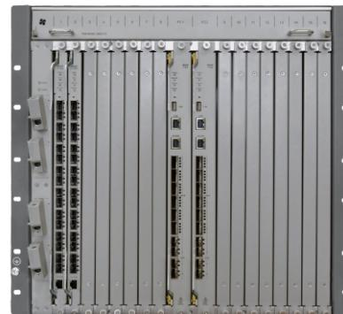
The system may contain one or two MA5K-FC64 core switch modules. Installing two modules allows to build a highly reliable system by providing switch redundancy and increasing system bandwidth by distributing data streams between modules through stacking. The modules interact via 100 Gbps interfaces operating in load sharing and redundancy modes.
