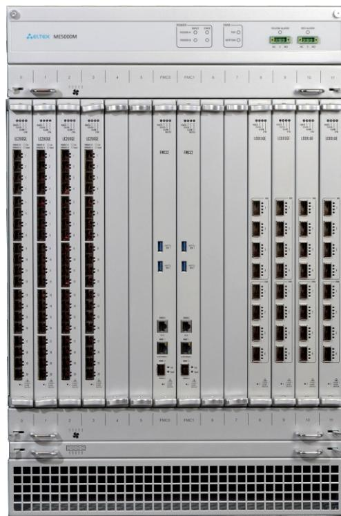
Fault tolerance of the device is ensured by redundant power supply (the chassis has two DC-48V power inputs and a distributed power supply scheme) and the use of replaceable fan modules. All replaceable modules, including management and switching boards, line cards, and fan modules, can be replaced while the unit is running.
