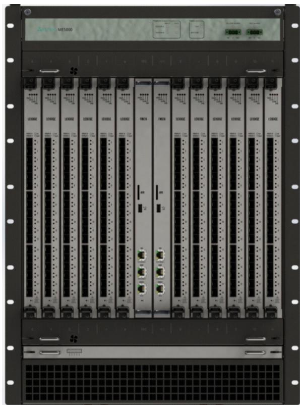
Fault tolerance of the device is ensured by redundant power supply (the chassis has two DC-48V power inputs and a distributed power supply scheme) and the use of replaceable fan modules. All replaceable modules, including management and switching boards, line cards, and fan modules, can be replaced while the unit is running.
