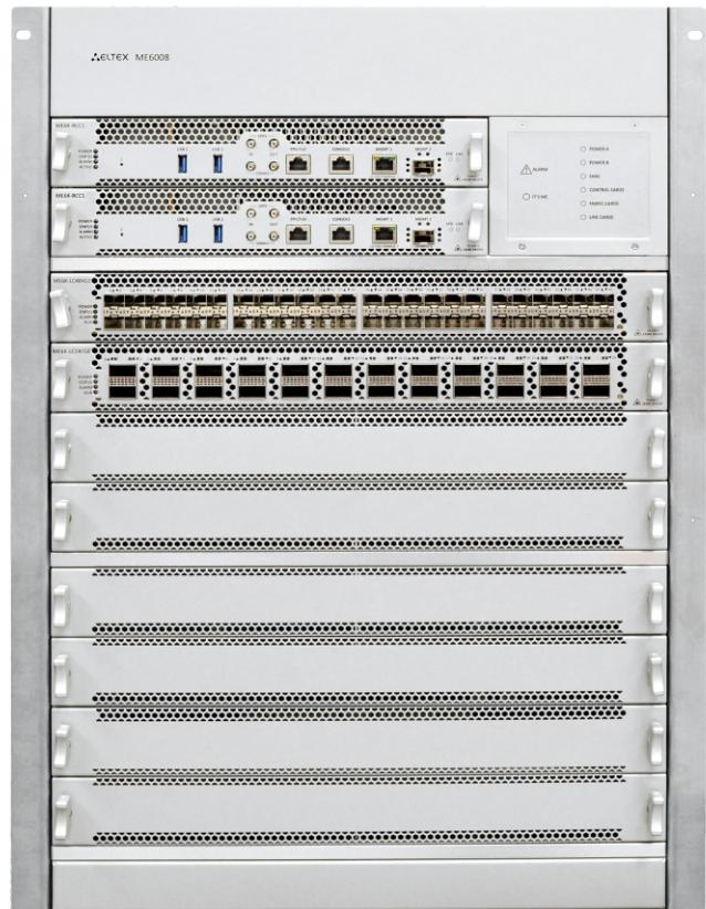
All redundant units including switch and management cards, line cards, and fan modules are hot-swappable.
